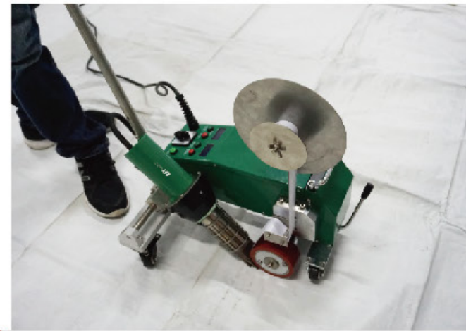
Tape Welding of Tarpaulin LST-MAT2
